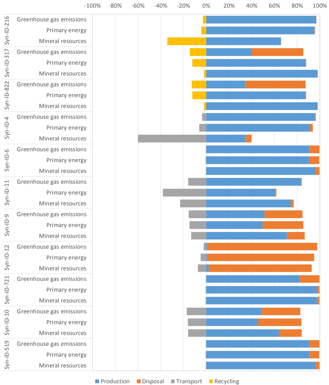
Fig. 3.9: Comparison of carbon, primary energy and mineral resource savings categories for all synergies divided into the contribution from avoided production, avoided disposal, additional transport and additional recycling
